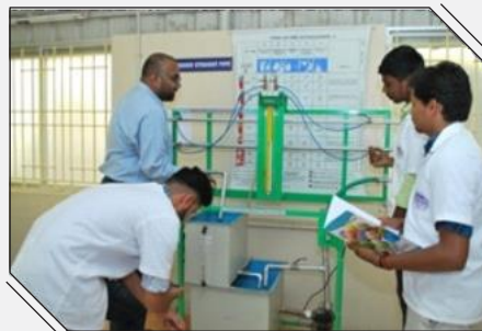
Faculty demonstrating on Flow through Straight pipe Experiment to students in Fluid Mechanics Laboratory
