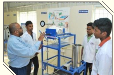
Faculty demonstrating on Plate and Frame Filter Press Experiment to students in Mechanical Operations Laboratory
