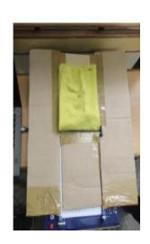
The T-shirt is placed on the folding platform of the T-shirt folding machine. The Arduino receives a signal to begin folding the T-shirt when the switch is pressed in its presence. To fold the T-shirt methodically, the Arduino gives the servo motors precise movements to follow. The machine may release the folded T-shirt after the folding process is finished, readying it for storage or exhibition.
