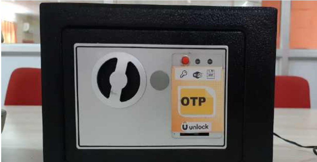
FIGURE B 9.4.3gOTP Based Security Locker
