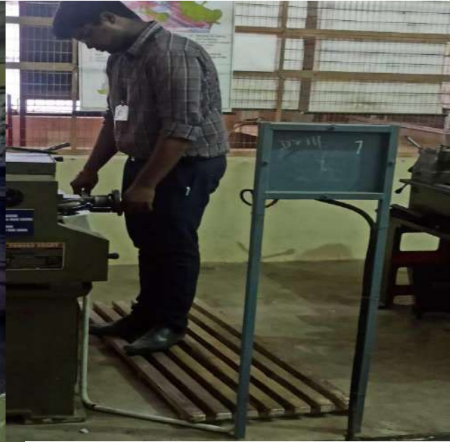
Figure B. 6.3b Safety platforms in lathe
