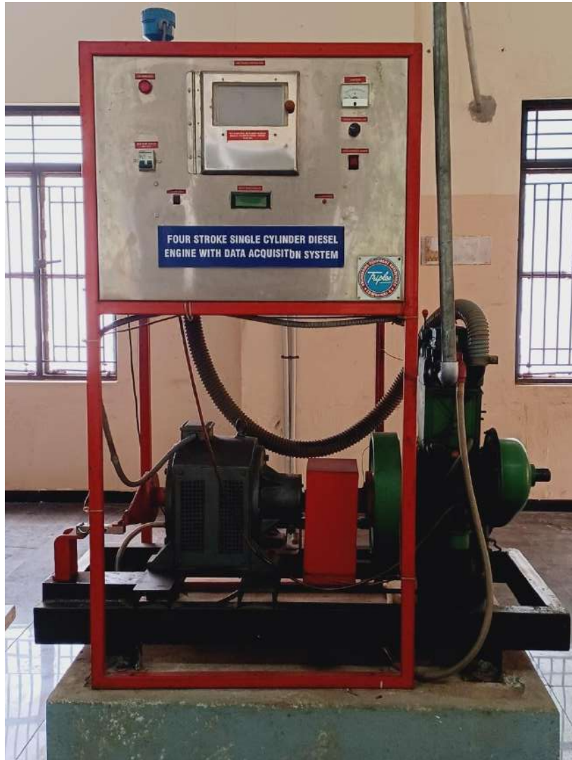
Fig B 5.8.3f Four stroke Single cylinder Diesel Engine with Data Acquisition system
